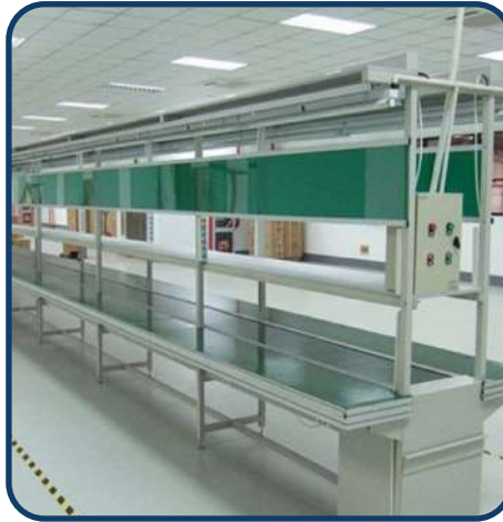
FLAT BELT CONVEYOR WITH SIDE WORKING PLATFORM
