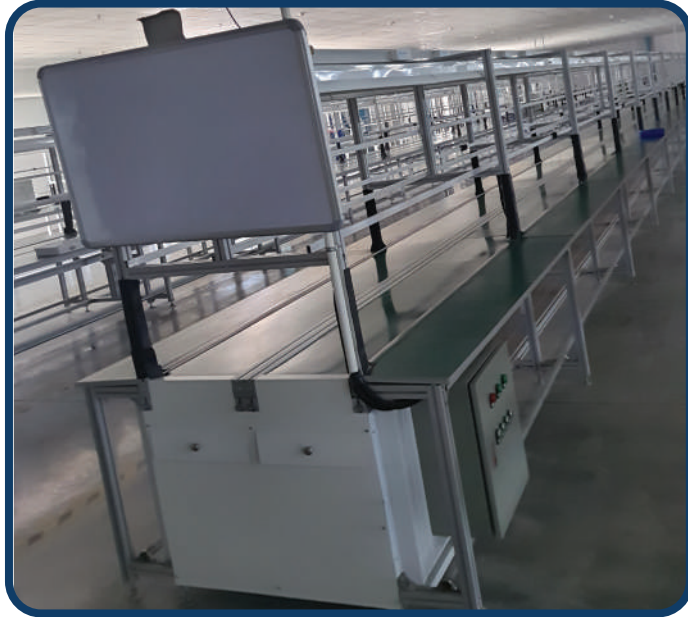
MAIN ASSEMBLY CONVEYOR
