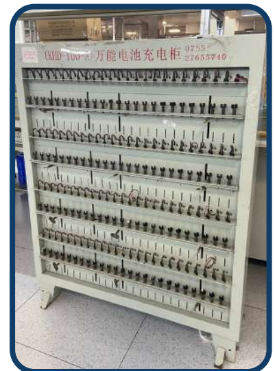
BATTERY AGING/ CHARGING TROLLEY
